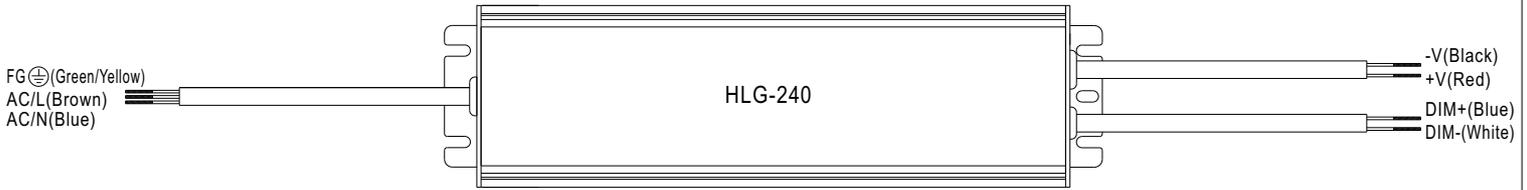
※ Built-in 3 in 1 dimming function, IP67 rated. Output constant current level can be adjusted through output cable by connecting a resistance or 1 ~ 10Vdc or 10V PWM signal between DIM+ and DIM-.
