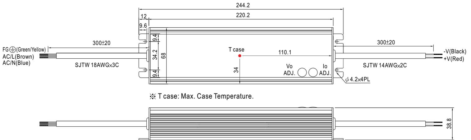
※ IP65 rated. Output voltage and constant current level can be adjusted through internal potentiometer.
