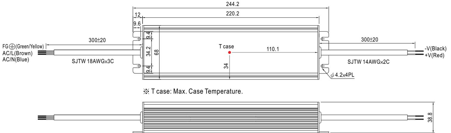
※IP67 rated. Cable for I/O connection.
